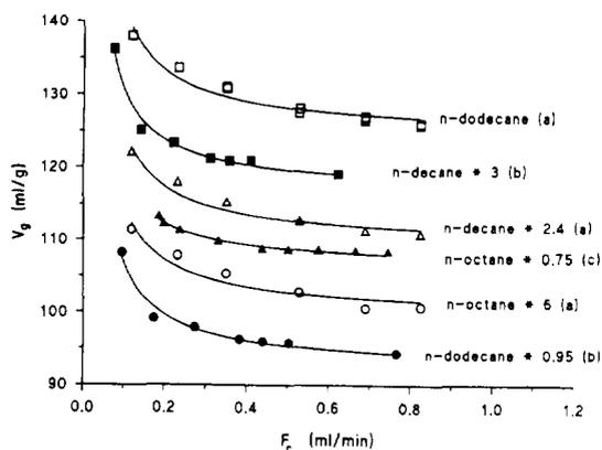
Fig. 1. Specific retention volumes of a few solutes at different flow-rates. Preliminary results. (a) Column 3 (Table 1), 120°C; (b) column 1, 160°C; (c) column 1, 80°C. Carrier gas, nitrogen. *n*-Decane \* 3, for example, means that the value of  $V_g$  of *n*-decane shown in the plot is three times the correct value.
