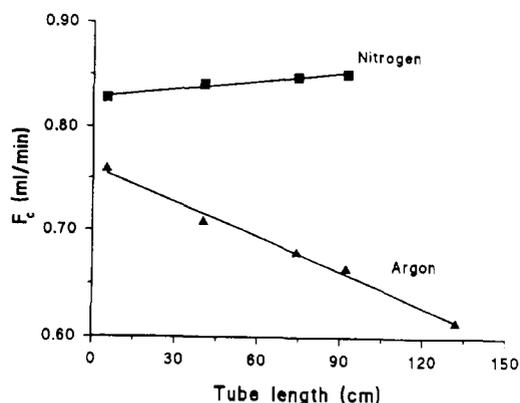
Fig. 3. Effect of the length of the polysiloxane connecting tube (chromatographic column–flow meter) on the experimentally measured flow-rate. Column 3, 120°C; inlet pressure for  $N_2$ , 173 kPa; inlet pressure for Ar, 186 kPa.
