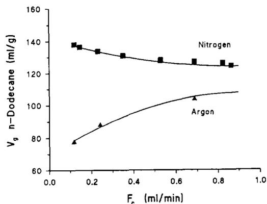
Fig. 2. Experimental specific retention volumes of *n*-dodecane on column 3 (TFPS35) at 120°C, with nitrogen and argon as carrier gases.
