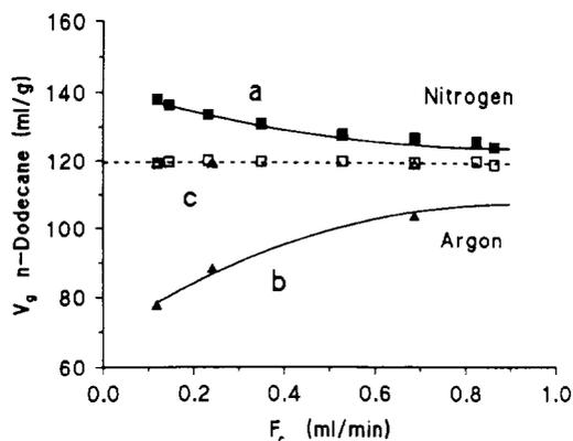
Fig. 4. Experimental specific retention volumes of *n*-dodecane on column 3 (TFPS35) at 120°C, with nitrogen and argon as carrier gases, obtained by applying Eq. 1 (curves a and b), and values obtained by applying Eq. 11 to the same set of experimental results using ( $\Delta$ ) argon and ( $\square$ ) nitrogen. Line c represents the average value of the specific retention volumes obtained with Eq. 11.
